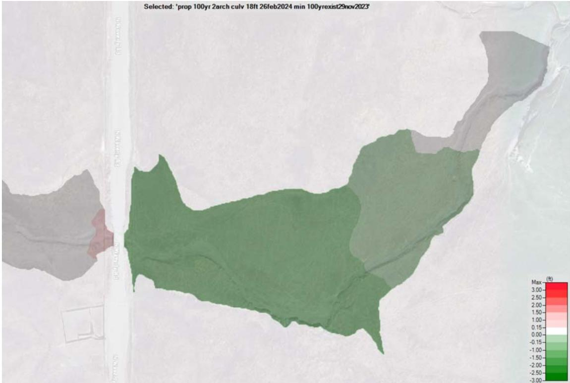
Figure 21: Water Surface elevation Comparison between existing and proposed conditions
