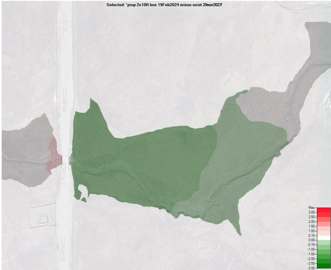
Figure 26: Water Surface elevation Comparison between existing and proposed conditions
