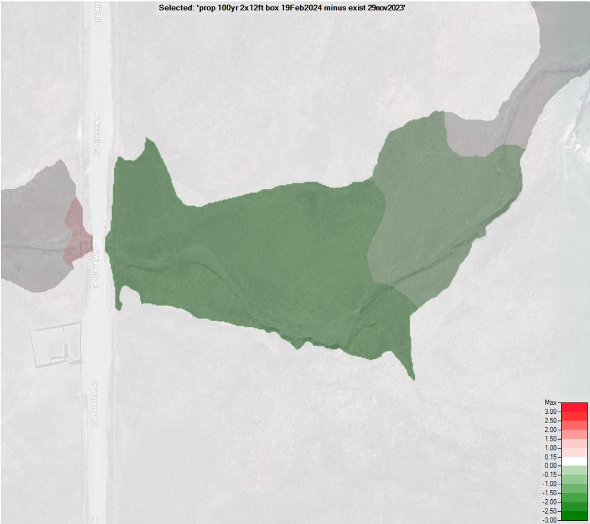
Figure 31: Water Surface Elevation Comparison between Existing and Proposed Conditions
