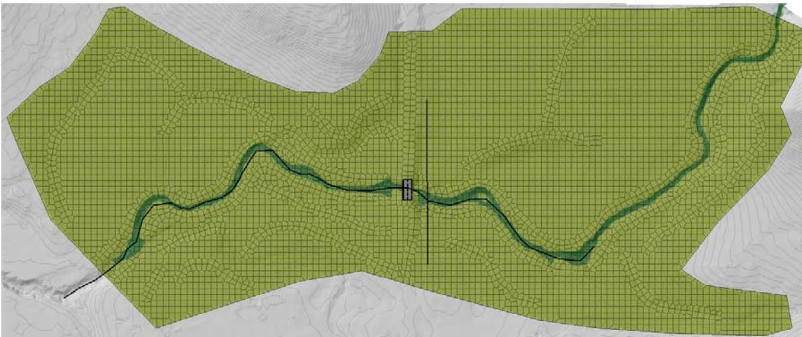
*Figure 5. The channel bottom is smooth with relatively low manning “n” value and the overbank areas are sparsely vegetated with relatively low manning “n” values.*
