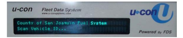
System will recognize key and identify vehicle. Display will request vehicle odometer reading, enter current odometer using keypad
