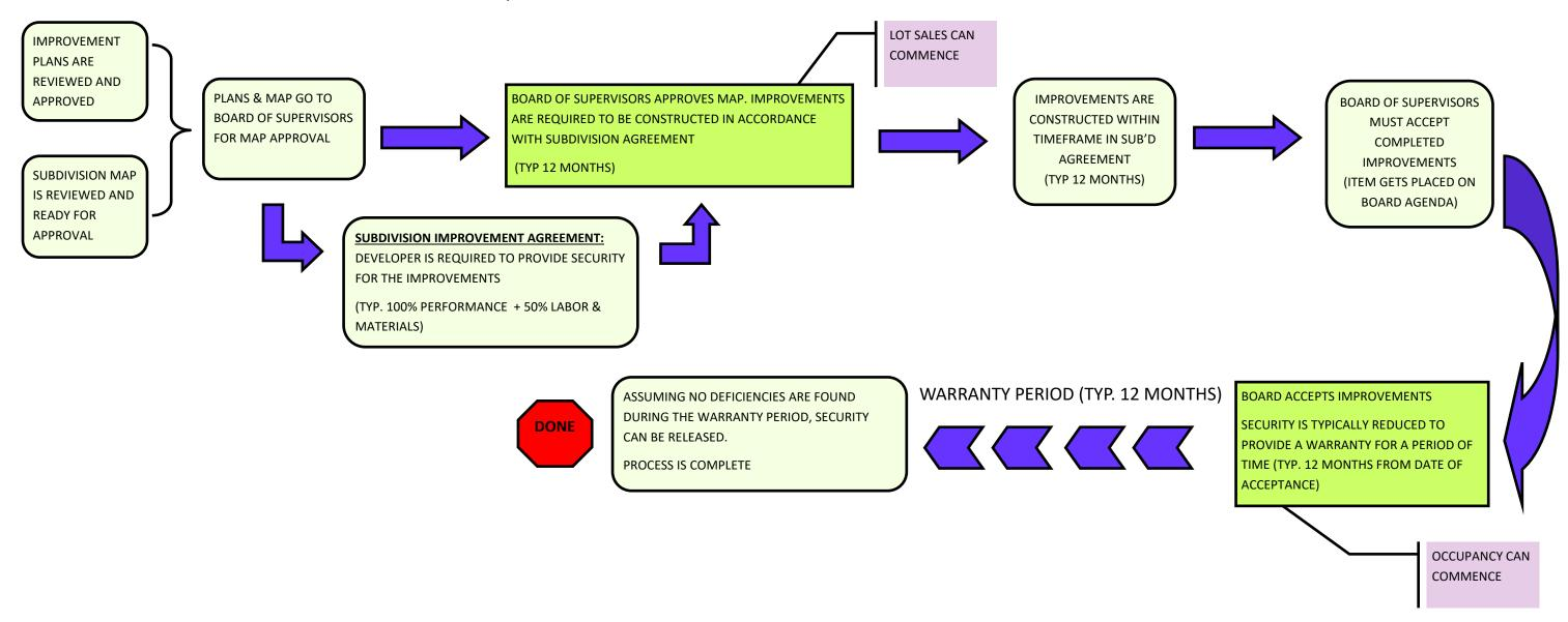
THIS DIAGRAM IS INTENDED TO PROVIDE A GENERAL OVERVIEW OF THE PROCESS AND DOES NOT ACCOUNT FOR UNIQUE OR SPECIAL CIRCUMSTANCES. REVIEW TIMES ARE NOT PROVIDED AND CAN VARY DUE TO A NUMBER OF FACTORS. CONSTRUCTION TIMEFRAMES CAN VARY DUE TO A NUMBER OF FACTORS. THE TIMELINE ASSOCIATED WITH PLACING ITEMS ON THE BOARD OF SUPERVISORS AGENDA IS TYPICALLY 1-2 MONTHS.
