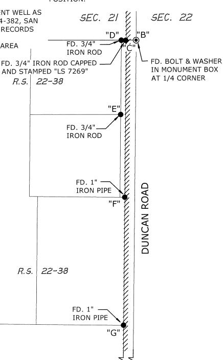
ANGLE AND DISTANCE TABLE BS DISTANCE FS DISTANCE BS-O-FS **ANGLE** A-C-B 90°35'46" 2645.41' 20.06' 2645.56 29.99 A-D-B 89°55'57" A-E-B 168°09'35" 23.25' 154.10' 320.53' A-F-B 175°55'53" 2325.87' A-G-B 177°27'33" 2065.79 580.35
