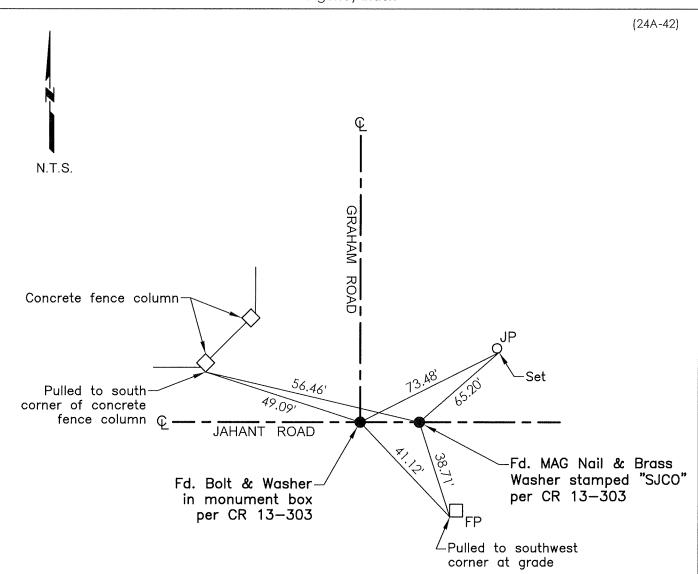
TR=Tree MB=Mailbox BM=Bench Mark EP=Edge of Pavement YL=Yellow Line FH=Fire Hydrant CR=Corner Record FP=Fence Post JP=Joint Pole LP=Light Pole PP=Power Pole GP=Guy Pole SP=Service Pole TP=Telephone Pole S.F.N.=Searched Found Nothing N.T.S.=Not To Scale M&P=Maps & Plats PM=Parcel Map RS=Record of Survey FB=Field Book N=North SDI=Storm Drain Inlet TOC=Top of Curb PCC=Portland Cement Concrete
