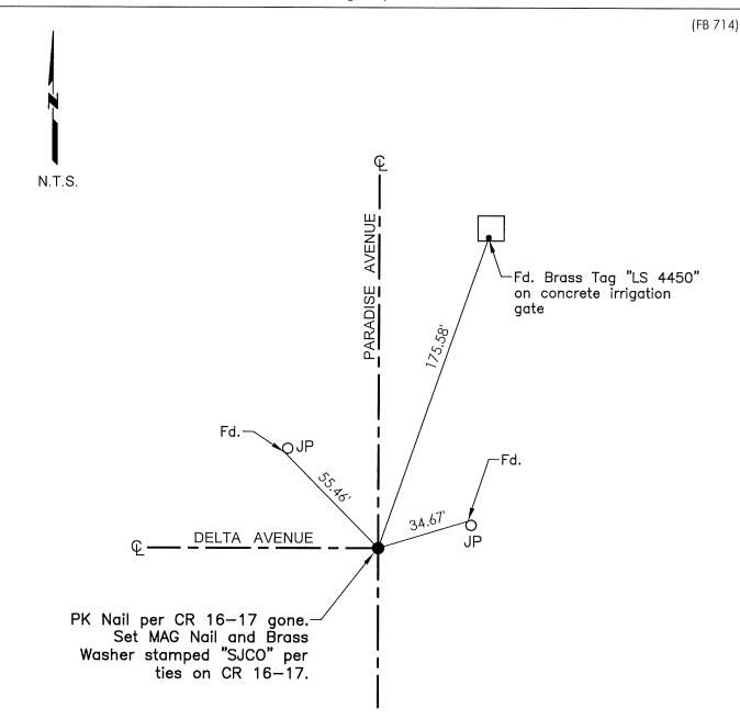
TR=Tree MB=Mailbox BM=Bench Mark EP=Edge of Pavement YL=Yellow Line FH=Fire Hydrant CR=Corner Record FP=Fence Post JP=Joint Pole LP=Light Pole PP=Power Pole GP=Guy Pole SP=Service Pole TP=Telephone Pole S.F.N.=Searched Found Nothing N.T.S.=Not To Scale M&P=Maps & Plats PM=Parcel Map RS=Record of Survey FB=Field Book N=North SDI=Storm Drain Inlet TOC=Top of Curb PCC=Portland Cement Concrete
