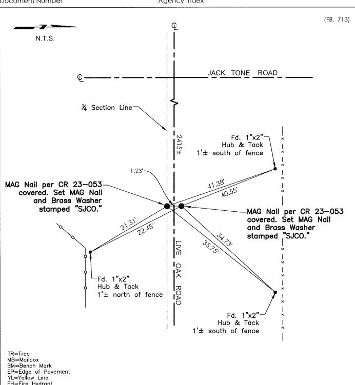
FH=Fire Hydrant CR=Corner Record FP=Fence Post JP=Joint Pole LP=Light Pole PP=Power Pole GP=Guy Pole SP=Service Pole TP=Telephone Pole S.F.N.=Searched Found Nothing N.T.S.=Not To Scale M&P=Maps & Plats PM=Parcel Map RS=Record of Survey FB=Field Book N=North SDI=Storm Drain Inlet TOC=Top of Curb PCC=Portland Cement Concrete
