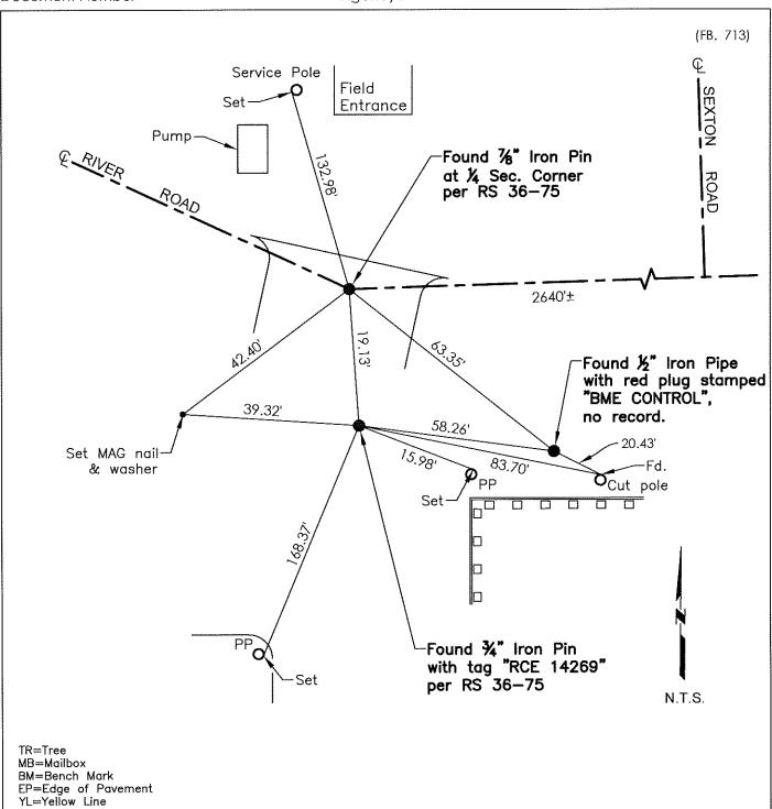
EP=Edge of Pavement YL=Yellow Line FH=Fire Hydrant CR=Corner Record FP=Fence Post JP=Joint Pole LP=Light Pole PP=Power Pole GP=Guy Pole SP=Service Pole TP=Telephone Pole S.F.N.=Searched Found Nothing N.T.S.=Not To Scale M&P=Maps & Plats PM=Parcel Map RS=Record of Survey FB=Field Book N=North SDI=Storm Drain Inlet TOC=Top of Curb PCC=Portland Cement Concrete
