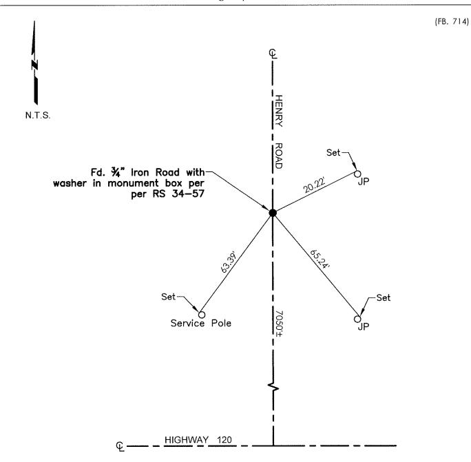
TR≔Tree MB=Mailbox BM=Bench Mark EP=Edge of Pavement YL=Yellow Line FH=Fire Hydrant CR=Corner Record FP=Fence Post JP=Joint Pole LP=Light Pole PP=Power Pole GP=Guy Pole SP=Service Pole TP=Telephone Pole S.F.N.=Searched Found Nothing N.T.S.=Not To Scale M&P=Maps & Plats PM=Parcel Map
