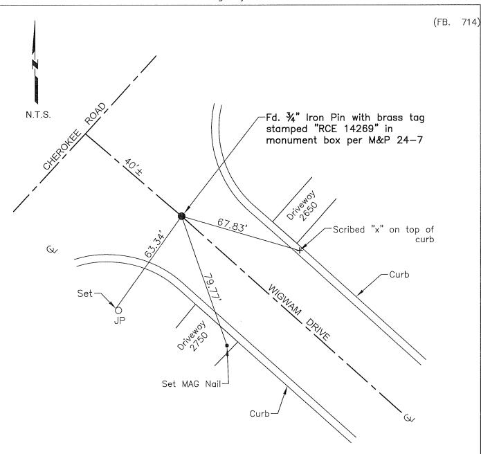
TR=Tree MB=Mailbox BM=Bench Mark EP=Edge of Pavement YL=Yellow Line FH=Fire Hydrant CR=Corner Record FP=Fence Post JP=Joint Pole LP=Light Pole PP=Power Pole GP=Guy Pole SP=Service Pole TP=Telephone Pole S.F.N.=Searched Found Nothing N.T.S.=Not To Scale M&P=Maps & Plats
