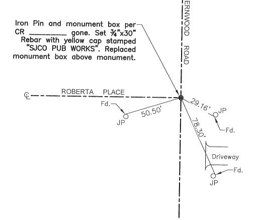
TR=Tree MB=Mailbox BM=Bench Mark EP=Edge of Pavement YL=Yellow Line FH=Fire Hydrant CR=Corner Record FP=Fence Post JP=Joint Pole LP=Light Pole PP=Power Pole GP=Guy Pole SP=Service Pole TP=Telephone Pole S.F.N.=Searched Found Nothing N.T.S.=Not To Scale M&P=Maps & Plats PM=Parcel Map RS=Record of Survey FB=Field Book N=North SDI=Storm Drain Inlet TOC=Top of Curb PCC=Portland Cement Concrete
