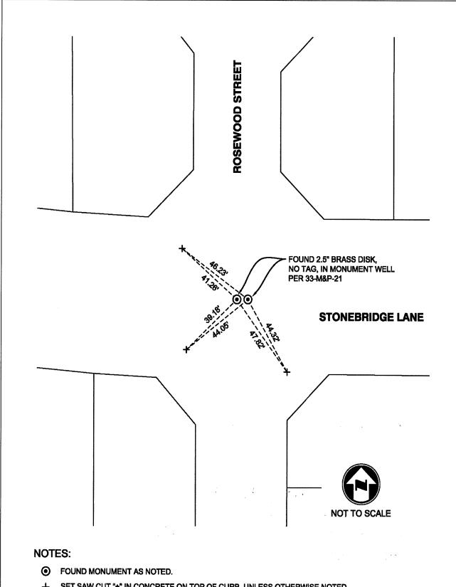
+ SET SAW CUT "+" IN CONCRETE ON TOP OF CURB, UNLESS OTHERWISE NOTED.
