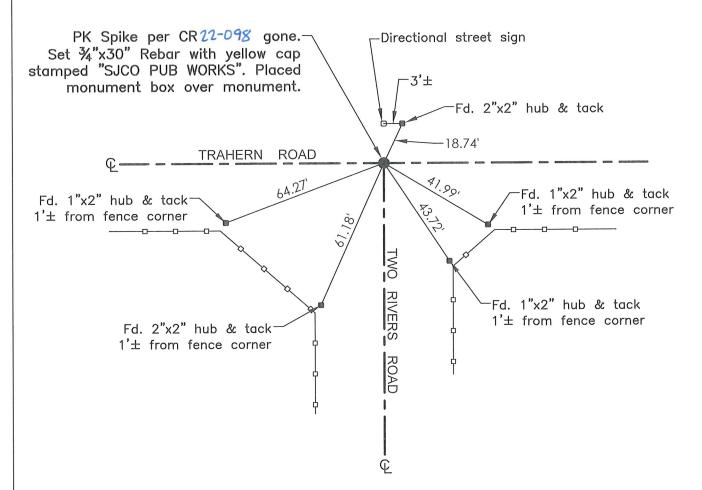
TR=Tree MB=Mailbox BM=Bench Mark EP=Edge of Pavement YL=Yellow Line FH=Fire Hydrant CR=Corner Record FP=Fence Post JP=Joint Pole LP=Light Pole PP=Power Pole GP=Guy Pole SP=Service Pole TP=Telephone Pole S.F.N.=Searched Found Nothing N.T.S.=Not To Scale M&P=Maps & Plats PM=Parcel Map RS=Record of Survey FB=Field Book N=North SDI=Storm Drain Inlet TOC=Top of Curb PCC=Portland Cement Concrete
