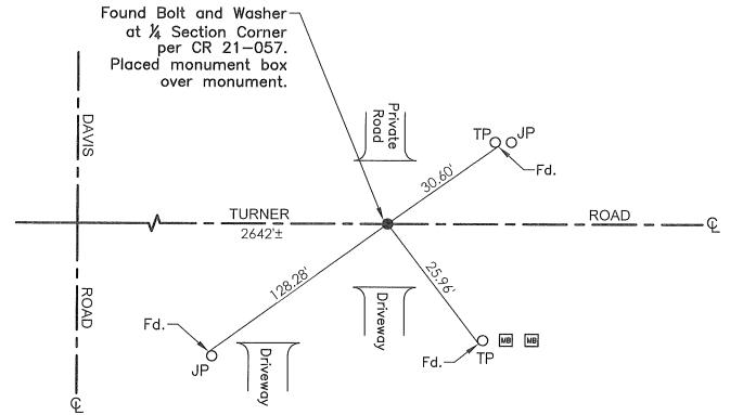
TR=Tree MB=Mailbox BM=Bench Mark EP=Edge of Pavement YL=Yellow Line FH=Fire Hydrant CR=Corner Record FP=Fence Post JP=Joint Pole LP=Light Pole PP=Power Pole GP=Guy Pole SP=Service Pole TP=Telephone Pole S.F.N.=Searched Found Nothing N.T.S.=Not To Scale M&P=Maps & Plats PM=Parcel Map RS=Record of Survey FB=Field Book N=North SDI=Storm Drain Inlet TOC=Top of Curb PCC=Portland Cement Concrete
