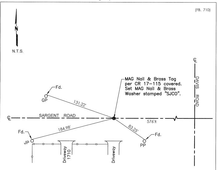
TR=Tree MB=Mailbox BM=Bench Mark EP=Edge of Pavement YL=Yellow Line FH=Fire Hydrant CR=Corner Record FP=Fence Post JP=Joint Pole LP=Light Pole PP=Power Pole GP=Guy Pole SP=Service Pole TP=Telephone Pole S.F.N.=Searched Found Nothing N.T.S.=Not To Scale M&P=Maps & Plats PM=Parcel Map RS=Record of Survey FB=Field Book N=North SDI=Storm Drain Inlet TOC=Top of Curb PCC=Portland Cement Concrete
