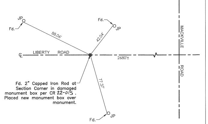
TR=Tree MB=Mailbox BM=Bench Mark EP=Edge of Pavement YL=Yellow Line FH=Fire Hydrant CR=Corner Record FP=Fence Post JP=Joint Pole LP=Light Pole PP=Power Pole GP=Guy Pole SP=Service Pole TP=Telephone Pole S.F.N.=Searched Found Nothing N.T.S.=Not To Scale M&P=Maps & Plats PM=Parcel Map RS=Record of Survey FB=Field Book N=North SDI=Storm Drain Inlet TOC=Top of Curb PCC=Portland Cement Concrete
