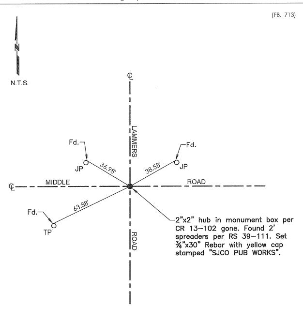
TR=Tree MB=Mailbox BM=Bench Mark EP=Edge of Pavement YL=Yellow Line FH=Fire Hydrant CR=Corner Record FP=Fence Post JP=Joint Pole LP=Light Pole PP=Power Pole GP=Guy Pole SP=Service Pole TP=Telephone Pole S.F.N.=Searched Found Nothing N.T.S.=Not To Scale M&P=Maps & Plats PM=Parcel Map RS=Record of Survey FB=Field Book N=North SDI=Storm Drain Inlet TOC=Top of Curb PCC=Portland Cement Concrete
