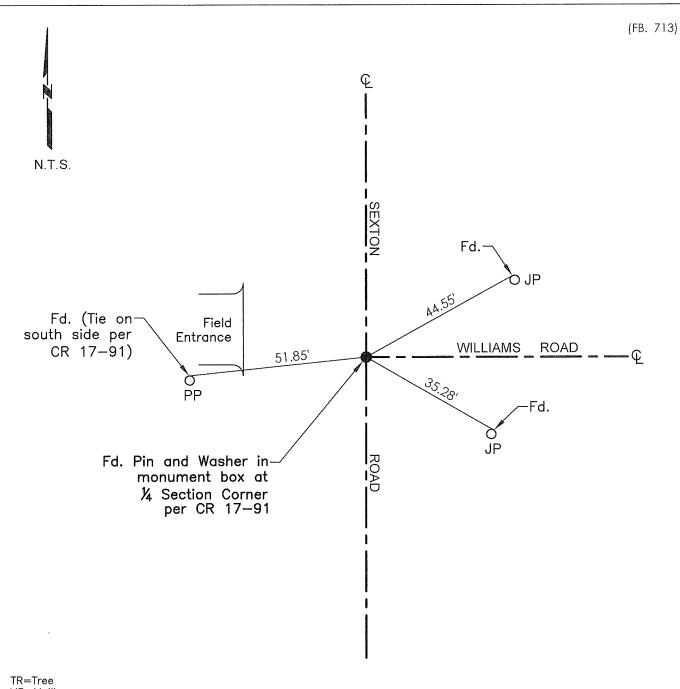
MB=Mailbox BM=Bench Mark EP=Edge of Pavement YL=Yellow Line FH=Fire Hydrant CR=Corner Record FP=Fence Post JP=Joint Pole LP=Light Pole PP=Power Pole GP=Guy Pole SP=Service Pole TP=Telephone Pole S.F.N.=Searched Found Nothing N.T.S.=Not To Scale M&P=Maps & Plats PM=Parcel Map RS=Record of Survey FB=Field Book N=North SDI=Storm Drain Inlet TOC=Top of Curb PCC=Portland Cement Concrete
