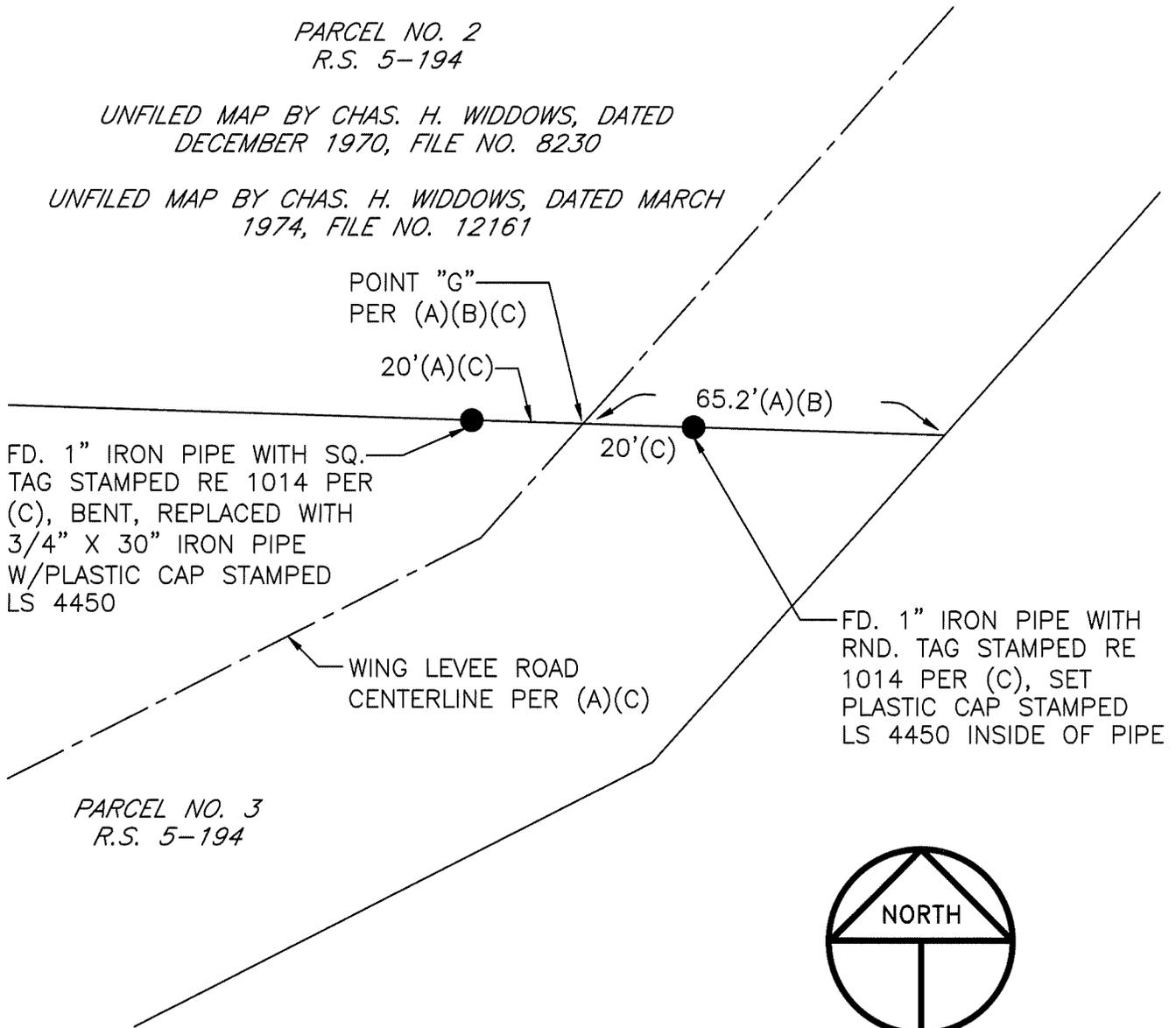
FD. 1" IRON PIPE WITH SQ. TAG STAMPED RE 1014 PER (C), BENT, REPLACED WITH 3/4" X 30" IRON PIPE W/PLASTIC CAP STAMPED LS 4450
