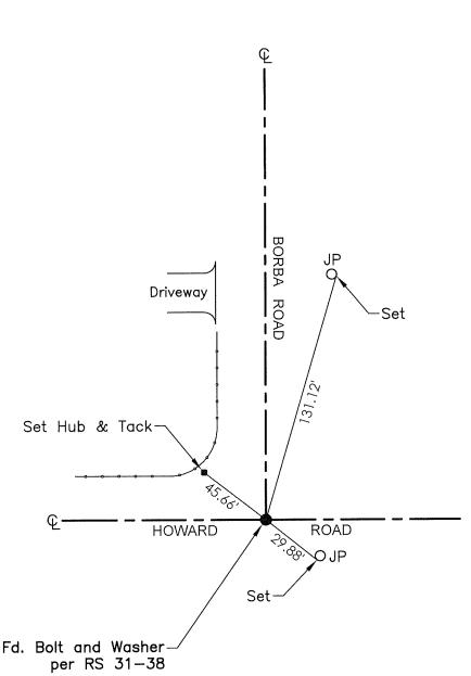
TR=Tree MB=Mailbox BM=Bench Mark EP=Edge of Pavement YL=Yellow Line FH=Fire Hydrant CR=Corner Record FP=Fence Post JP=Joint Pole LP=Light Pole PP=Power Pole GP=Guy Pole SP=Service Pole TP=Telephone Pole S.F.N.=Searched Found Nothing N.T.S.=Not To Scale M&P=Maps & Plats PM=Parcel Map RS=Record of Survey FB=Field Book N=North SDI=Storm Drain Inlet TOC=Top of Curb
