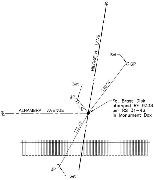
TR=Tree MB=Mailbox BM=Bench Mark EP=Edge of Pavement YL=Yellow Line FH=Fire Hydrant CR=Corner Record FP=Fence Post JP=Joint Pole LP=Light Pole PP=Power Pole GP=Guy Pole SP=Service Pole TP=Telephone Pole S.F.N.=Searched Found Nothing N.T.S.=Not To Scale M&P=Maps & Plats PM=Parcel Map RS=Record of Survey FB=Field Book N=North SDI=Storm Drain Inlet TOC=Top of Curb
