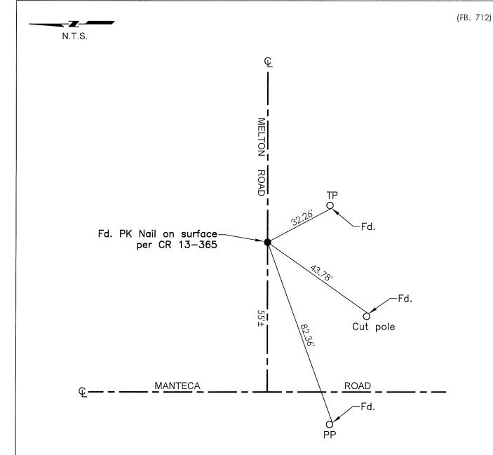
TR=Tree MB=Mailbox BM=Bench Mark EP=Edge of Pavement YL=Yellow Line FH=Fire Hydrant CR=Corner Record FP=Fence Post JP=Joint Pole LP=Light Pole PP=Power Pole GP=Guy Pole SP=Service Pole TP=Telephone Pole S.F.N.=Searched Found Nothing N.T.S.=Not To Scale M&P=Maps & Plats PM=Parcel Map RS=Record of Survey FB=Field Book N=North SDI=Storm Drain Inlet TOC=Top of Curb PCC=Portland Cement Concrete
