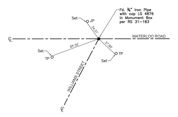
TR=Tree MB=Mailbox BM=Bench Mark EP=Edge of Pavement YL=Yellow Line FH=Fire Hydrant CR=Corner Record FP=Fence Post JP=Joint Pole LP=Light Pole PP=Power Pole GP=Guy Pole SP=Service Pole TP=Telephone Pole S.F.N.=Searched Found Nothing N.T.S.=Not To Scale M&P=Maps & Plats PM=Parcel Map RS=Record of Survey FB=Field Book N=North SDI=Storm Drain Inlet TOC=Top of Curb
