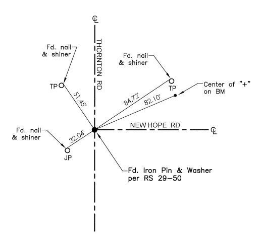
BM=Bench Mark FH=Fire Hydrant CR=Corner Record FP=Fence Post JP=Joint Pole LP=Light Pole PP=Power Pole GP=Guy Pole SP=Service Pole TP=Telephone Pole S.F.N.=Searched Found Nothing N.T.S.=Not To Scale M&P=Maps & Plats PM=Parcel Map RS=Record of Survey FB=Field Book N=North SDI=Storm Drain Inlet TOC=Top of Curb PCC=Portland Cement Concrete
