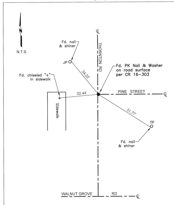
BM=Bench Mark FH=Fire Hydrant CR=Corner Record FP=Fence Post JP=Joint Pole LP=Light Pole PP=Power Pole GP=Guy Pole SP=Service Pole TP=Telephone Pole S.F.N.=Searched Found Nothing N.T.S.=Not To Scale M&P=Maps & Plats PM=Parcel Map RS=Record of Survey FB=Field Book N=North SDI=Storm Drain Inlet TOC=Top of Curb PCC=Portland Cement Concrete
