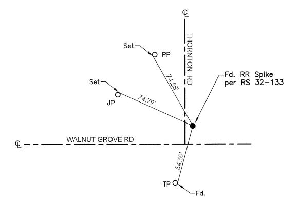
BM=Bench Mark FH=Fire Hydrant CR=Corner Record FP=Fence Post JP=Joint Pole LP=Light Pole PP=Power Pole GP=Guy Pole SP=Service Pole TP=Telephone Pole S.F.N.=Searched Found Nothing N.T.S.=Not To Scale M&P=Maps & Plats PM=Parcel Map RS=Record of Survey FB=Field Book N=North SDI=Storm Drain Inlet TOC=Top of Curb PCC=Portland Cement Concrete
