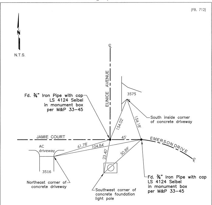
FH=Fire Hydrant CR=Corner Record FP=Fence Post JP=Joint Pole LP=Light Pole PP=Power Pole GP=Guy Pole SP=Service Pole TP=Telephone Pole S.F.N.=Searched Found Nothing N.T.S.=Not To Scale M&P=Maps & Plats PM=Parcel Map RS=Record of Survey FB=Field Book N=North SDI=Storm Drain Inlet TOC=Top of Curb PCC=Portland Cement Concrete
