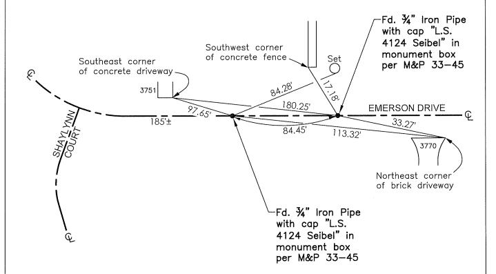
FH=Fire Hydrant CR=Corner Record FP=Fence Post JP=Joint Pole LP=Light Pole PP=Power Pole GP=Guy Pole SP=Service Pole TP=Telephone Pole S.F.N.=Searched Found Nothing N.T.S.=Not To Scale M&P=Maps & Plats PM=Parcel Map RS=Record of Survey FB=Field Book N=North SDI=Storm Drain Inlet TOC=Top of Curb PCC=Portland Cement Concrete
