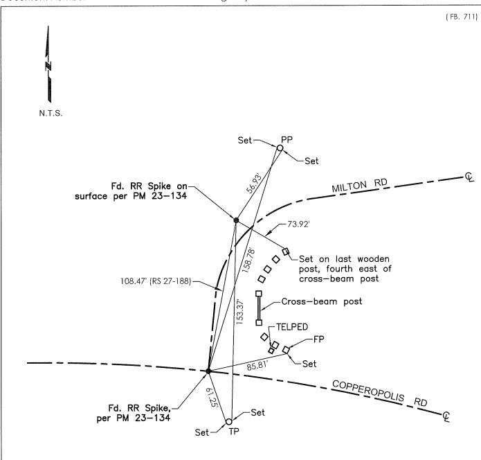
TR=Tree MB=Mailbox BM=Bench Mark EP=Edge of Pavement YL=Yellow Line FH=Fire Hydrant CR=Corner Record FP=Fence Post JP=Joint Pole LP=Light Pole PP=Power Pole GP=Guy Pole SP=Service Pole TP=Telephone Pole S.F.N.=Searched Found Nothing N.T.S.=Not To Scale
