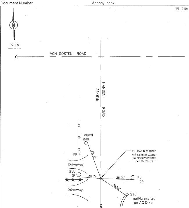
CR=Corner Record FP=Fence Post JP=Joint Pole LP=Light Pole PP=Power Pole GP=Guy Pole SP=Service Pole TP=Telephone Pole
