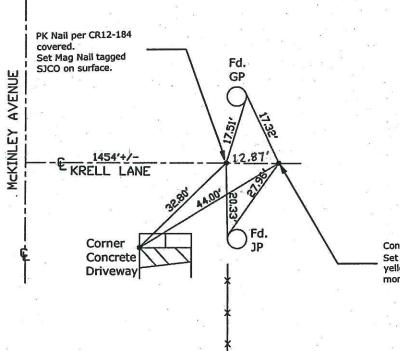
Concrete Nail per CR12-184 covered. Set ¾" x 30" rebar with yellow cap stamped SJCO in monument box.
