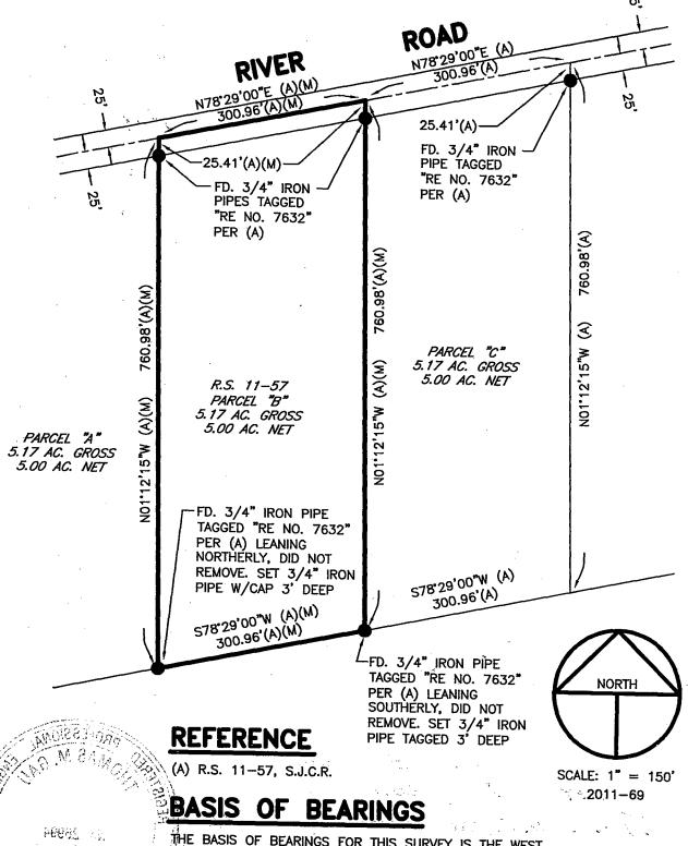
THE BASIS OF BEARINGS FOR THIS SURVEY IS THE WEST LINE OF PARCEL "B", SHOWN ON R.S. 11-57, S.J.C.R. AS N.01°12'15"W.
