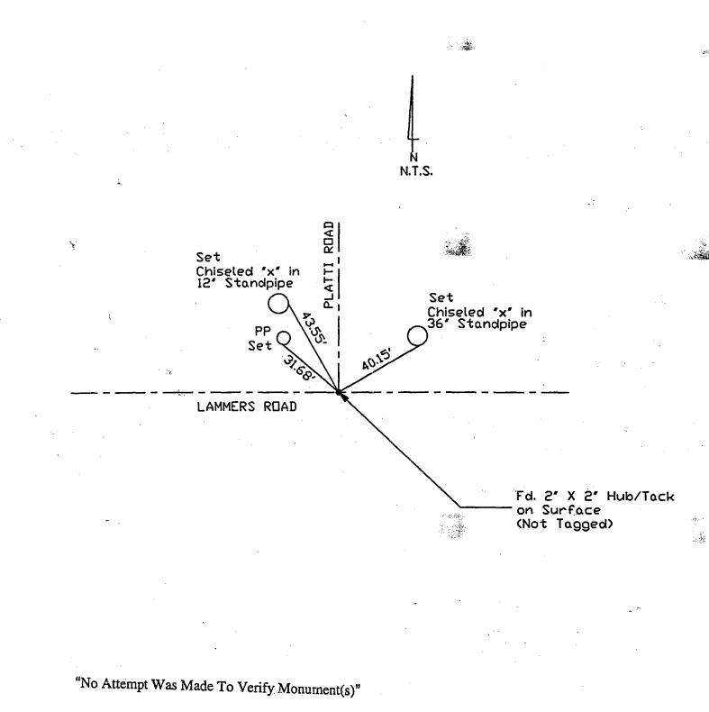
FP = Fence Post GP = Guy Post JP = Joint Pole PP = Power Pole SP = Service Pole TP = Telephone Pole N.T.S. = Not To Scale Set = Conc. Nails with Brass Wosher
