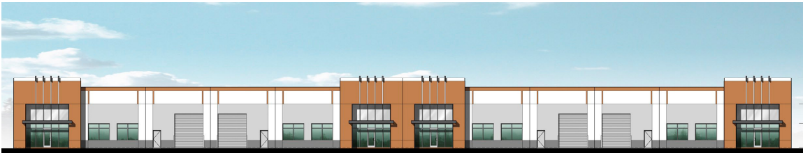
Figure 4.3.2 Clear entry demarcation and integrated loading doors
