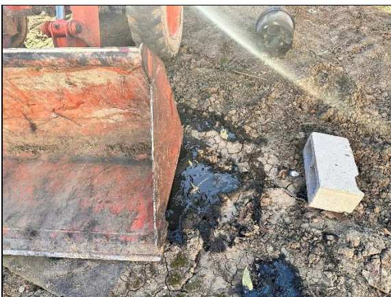
Photograph 17: View of Petroleum Leaking Out of Tractor South of Shop Area.
