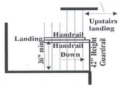
Stairways and landings are required to be a minimum of 36" in width. Handrails are required on at least one side of stairways with four or more risers, and continuous for the full length of the flight.
