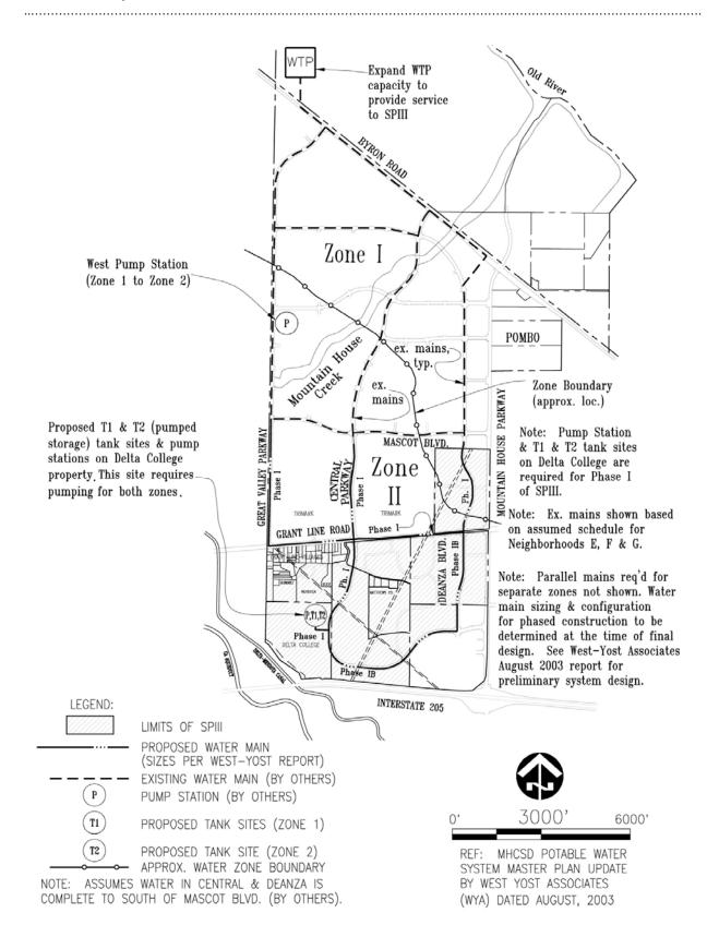
FIGURE 12-1: SPECIFIC PLAN III POTABLE WATER FACILITIES
