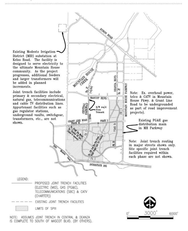
FIGURE 8-1: JOINT TRENCH FACILITIES FOR PRIMARY AND SECONDARY ELECTRICAL, NATURAL GAS, TELECOMMUNICATIONS, AND CABLE TV DISTRIBUTION LINES
