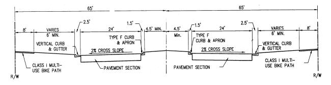
FIGURE 9-1: CENTRAL PARKWAY CROSS SECTION Source: MHCSD Design Manual
