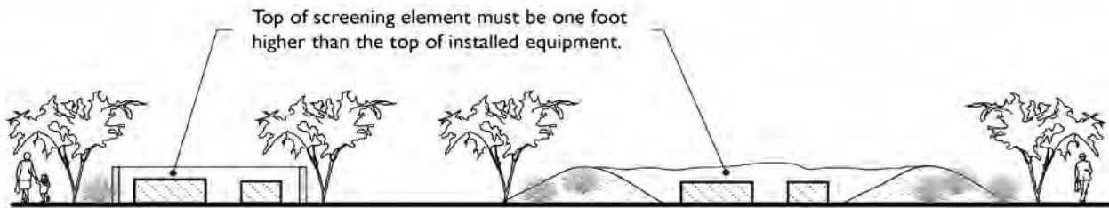
FIGURE 9-400.070-2: SCREENING OF GROUND MOUNTED EQUIPMENT
