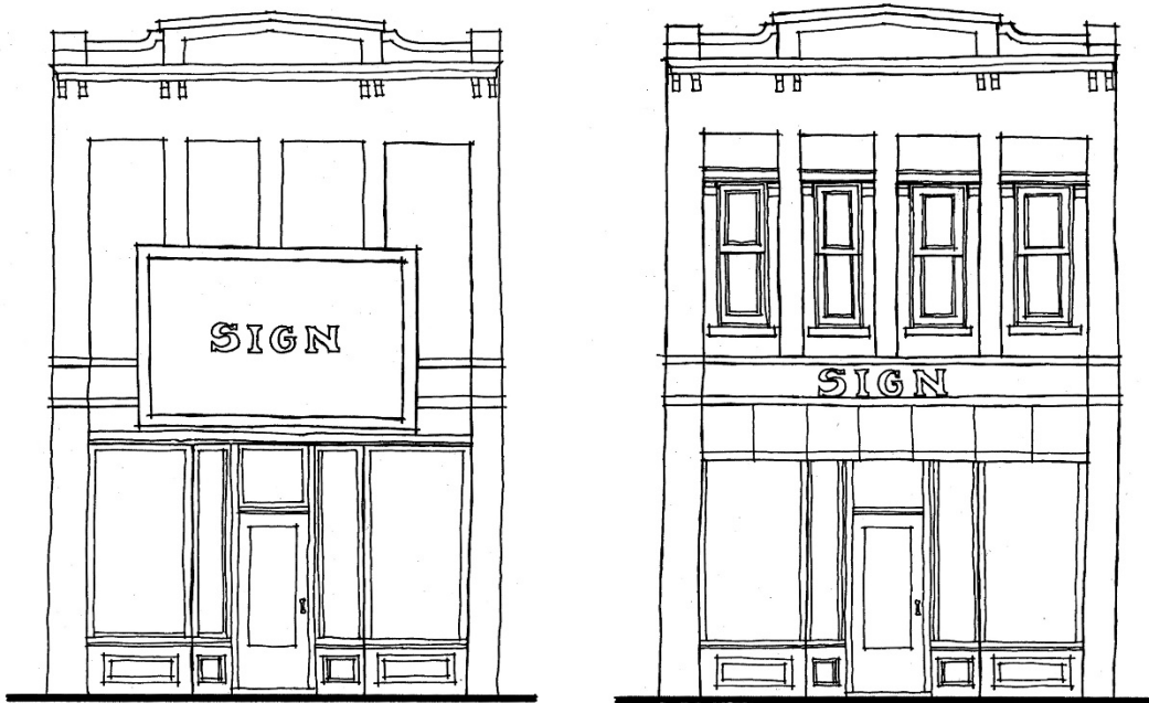
The sign on the left is an inappropriate use of sign size and placement. The sign on the right is the preferred sign size and placement.
